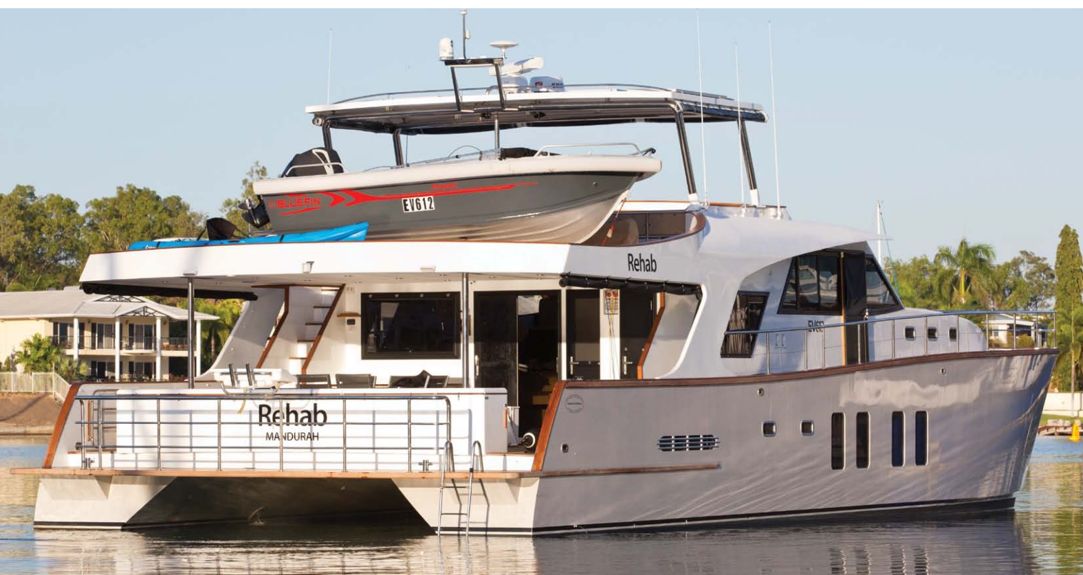
below: Pilothouse top blends into upper aft deck to provide shade and shelter.
