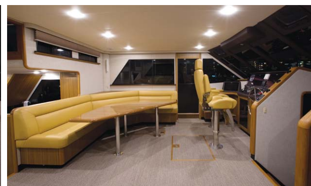
far left: Drive station is laid out in such a way as to be easy to access when docking yet comfortable for helmsman and navigator on passages.
